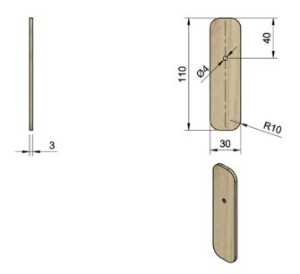
(Requires an M4 x 30 mm screw with a self-locking nut and two washers)
