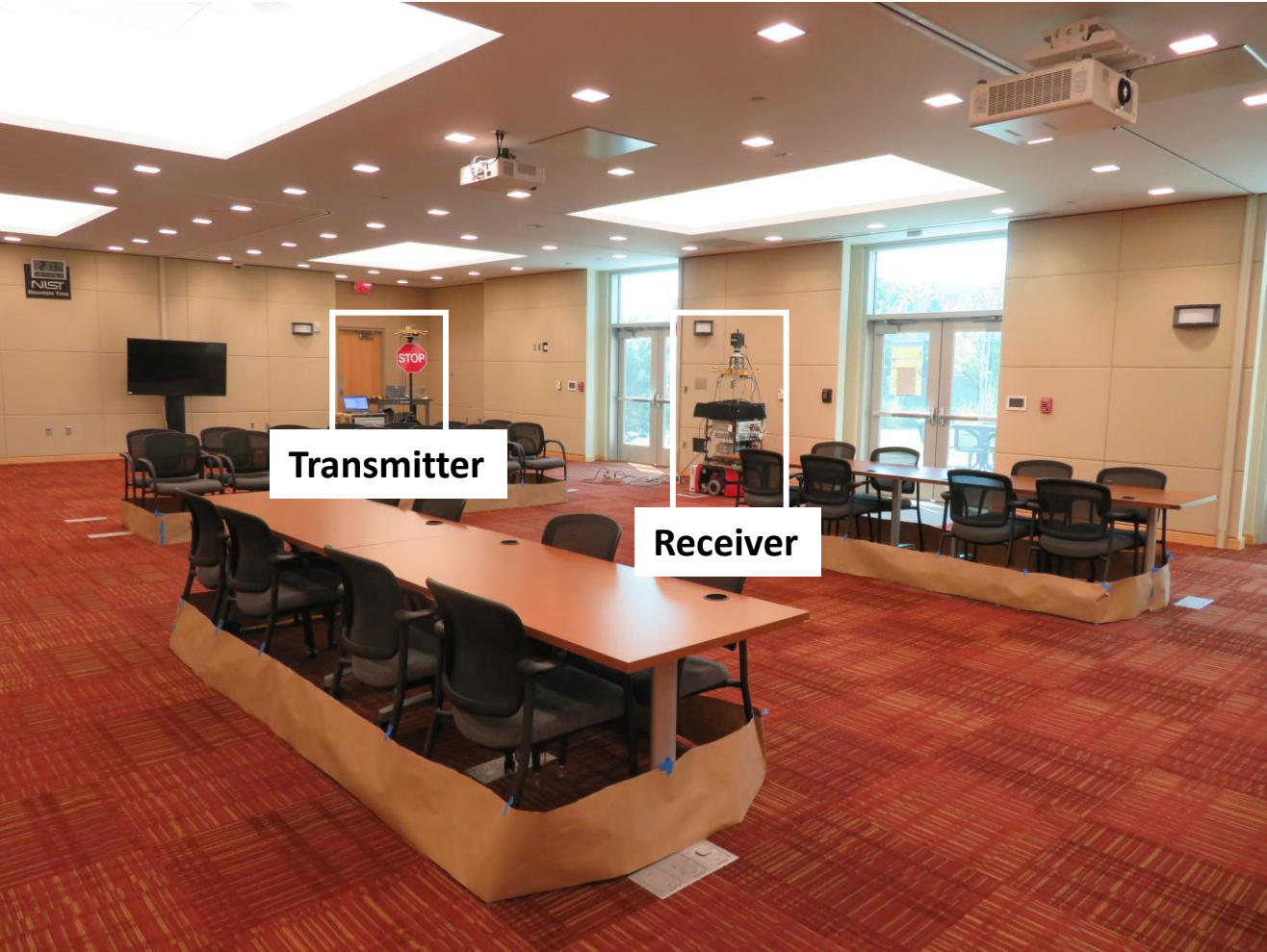
The transmitter was fixed in the corner of the room, while the receiver was moving in three areas across the room. 14
